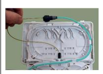
• Insert the BFU into the 6 x 3mm connector and Locking Tube until all the slack is taken up
