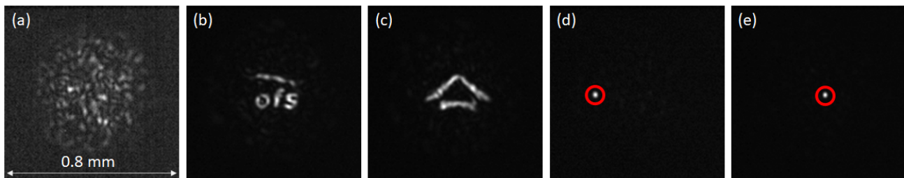
Figure 2. (a-e) Goal images produced at the distal end of OFS TCU-ME050H fiber calibrated with 45x45 spots. Images show the fiber core at approximately 13x magnification. Panel(a) shows the distal result when all launch conditions are multiplexed together with constant amplitude to indicate the core size and location within the image frames.
